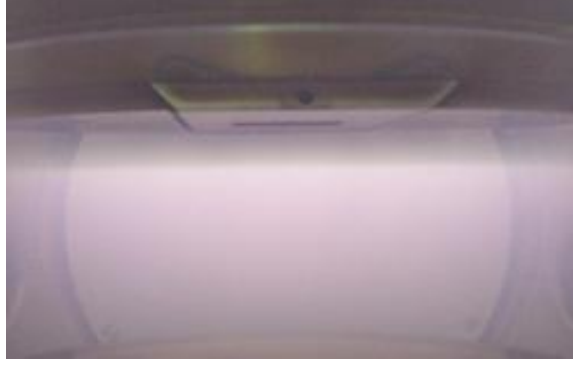
Figure 3.2: Photo of an ion sheath in front of a substrate to which an external voltage is applied. A dark zone is visible in front of the surface. The external voltage displaces the electrons there and thus also suppresses the light emission in this region.
