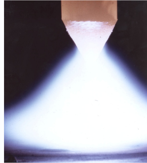
Example: argon arc at 1 atm
